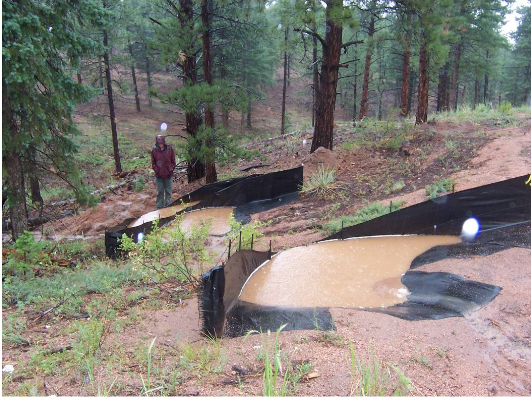
Figure 2.11. Excess storm runoff flowing over each of three sediment fences below a road segment at Spring Creek.
