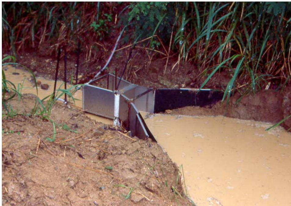
Figure 2b. Picture of a portable cutthroat flume similar to the one used to measure runoff from Maho-Road.
