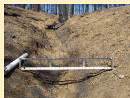
Figure 4. Pin frame used to measure rill incision.
