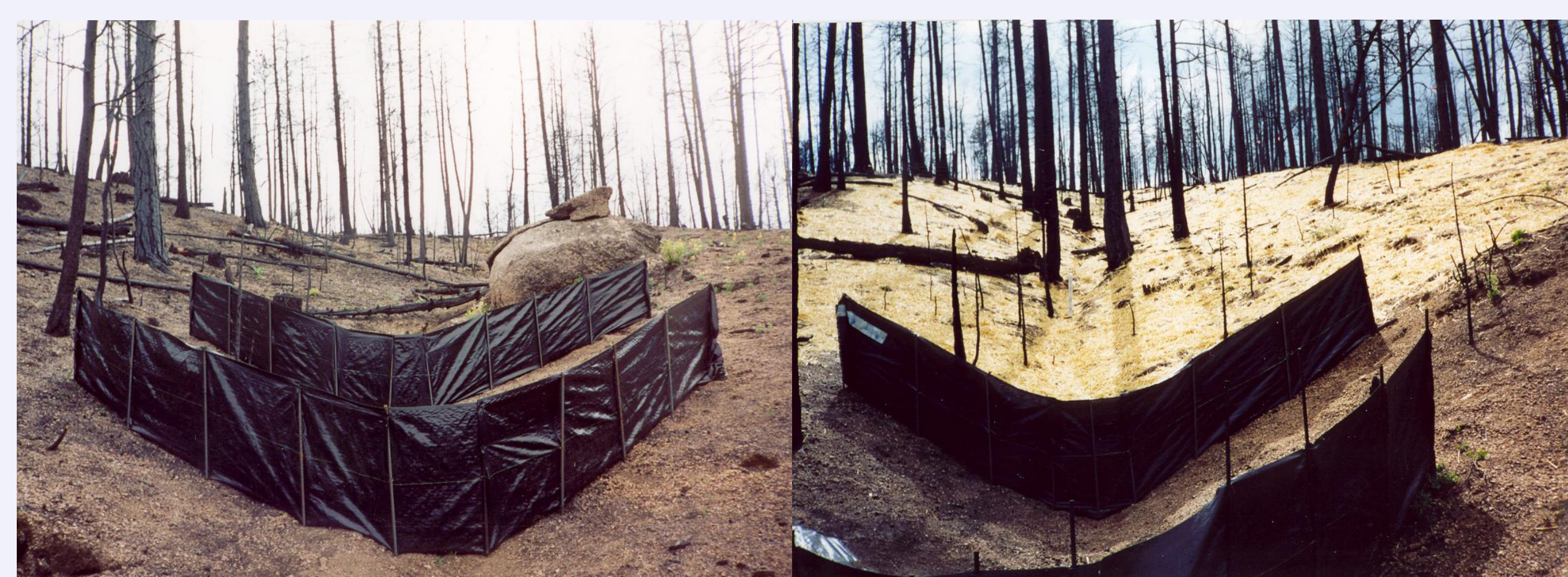
Figure 2. Paired swale design with adjacent control (left) and treated swales (right).
