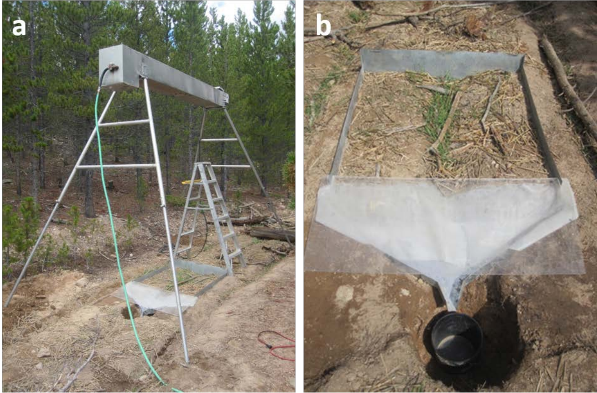
Figure 2.2. a) The Purdue-type rainfall simulator set up above a plot on a decommissioned road that had been ripped and mulched with wood strands and fertilizer. b) Detailed view of the plot prior to the rainfall simulation showing the central furrow, wood-strand mulch, and limited vegetative growth in the 10 months since the road had been treated.
