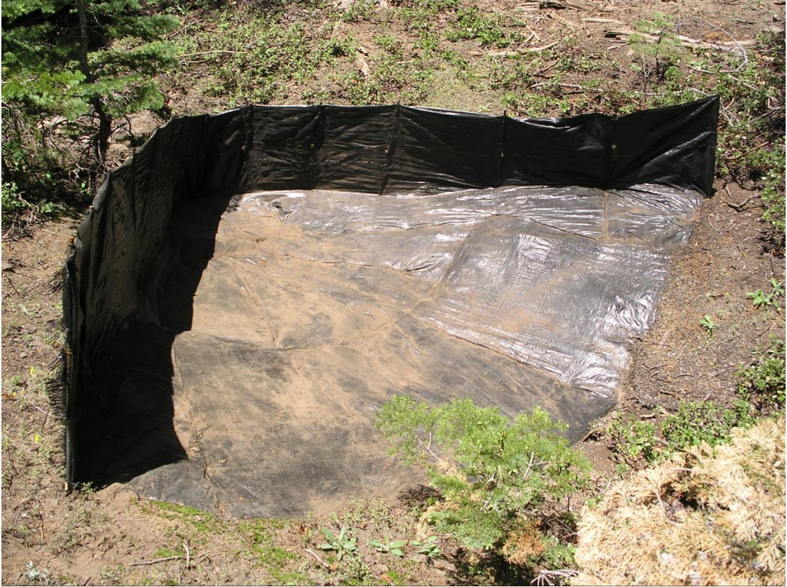
Figure 2.5. Sediment fences were installed on undisturbed, convergent swales in José Basin and the Providence Creek and Bull Creek watersheds. The fabric floor facilitates sediment removal and the accuracy of the measurement (photo by A. Korte).
