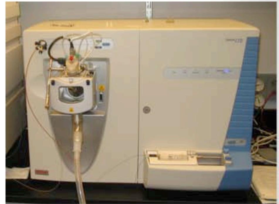
nanoLC-MS/MS (LTQ linear ion trap)
